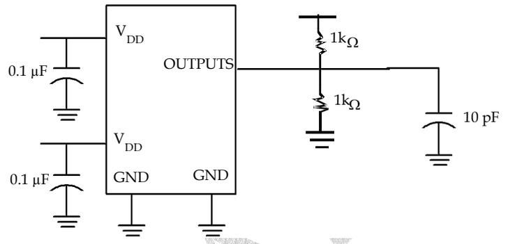
For parameter  $t_s$  (output slew rate) on -1H devices
